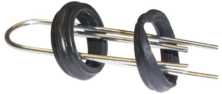
Before and After pics of the Injector seal due to oil pressure manifold O ring failure.
